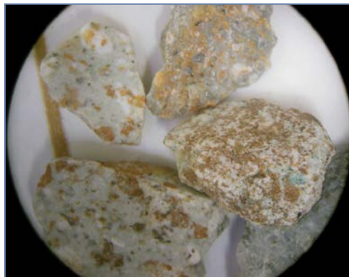
RC chips from historic drilling showing multiple sericitized porphyries and Cu-ox after sulfides
